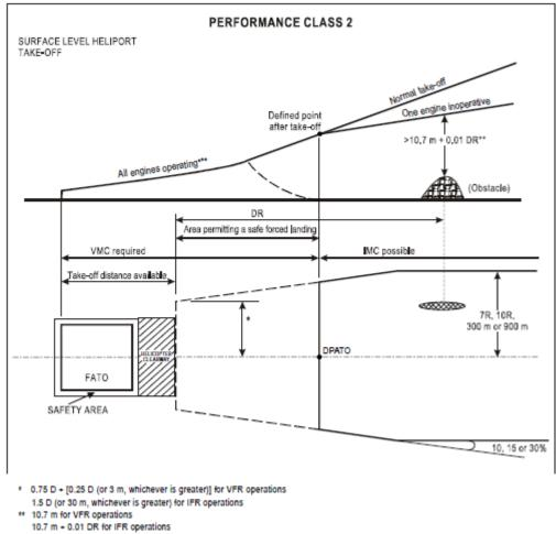
\*\*\* Only the all-engines-operating flight path is shown.
