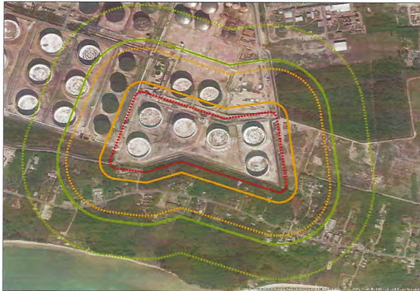
Figure A3.2 Effect distance of scenario 4.2 'Heavy fuel - tank pit (pool size 42.000 m 2 ) fire'.
