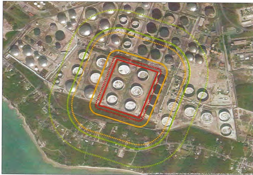
Figure A3.5 Effect distance of scenario 4.5 'Heavy fuel – tank pit (pool size 290 m x 290 m) fire'.
