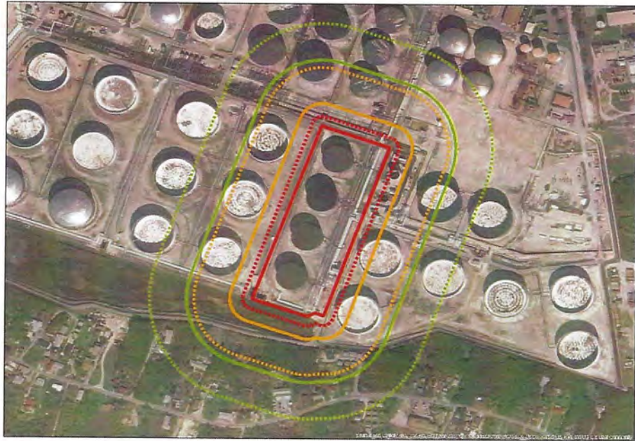
Figure A3.4 Effect distance of scenario 4.4 'Heavy fuel – tank pit (pool size 10.000 m 2 ) fire'.
