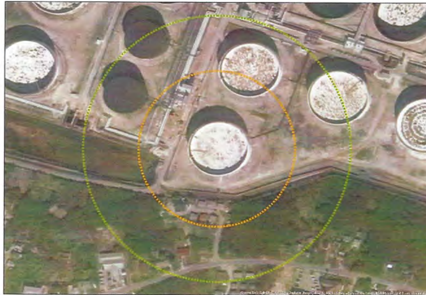
Figure A3.1: Effect distance of scenario 4.1 'Heavy fuel - tank fire'.
