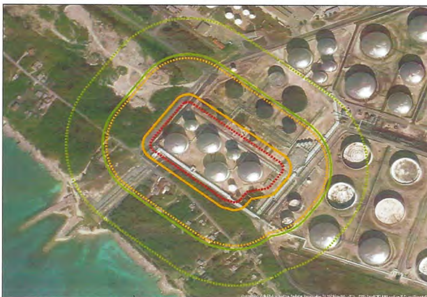
Figure A3.7 Effect distance of scenario 4.7 'Heavy fuel – tank pit (pool size 135 m x 135 m) fire'.
